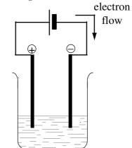
*Labels are not required.* one container, two electrodes, battery (and electrolyte);
